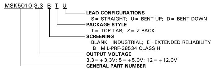
THE ABOVE EXAMPLE IS A  $\pm 3.3$ V, MILITARY REGULATOR USING THE TOP TAB PACKAGE WITH LEADS BENT UP.
