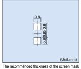
for soldering is between 100 and 150µm. The hole size of the screen mask should be same as the recommended land pattern or smaller.
