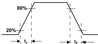
Figure 4. Output Rise and Fall Times
