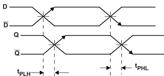
Figure 2. Propagation Delay
