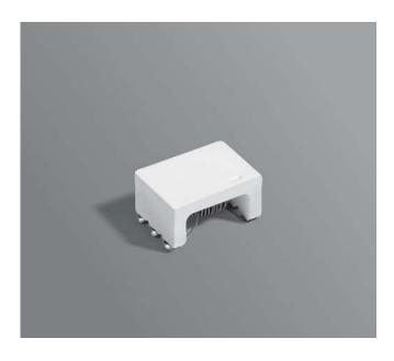
This low cost transformer is designed for use at 50 kHz to 300 kHz to sense continuous currents up to 3 Amps. The current windings can be connected in series to provide twice the output sensitivity. It offers 500 Vrms interwinding isolation.
