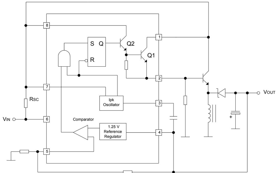
Voltage Inverting With External PNP Saturated Switch
