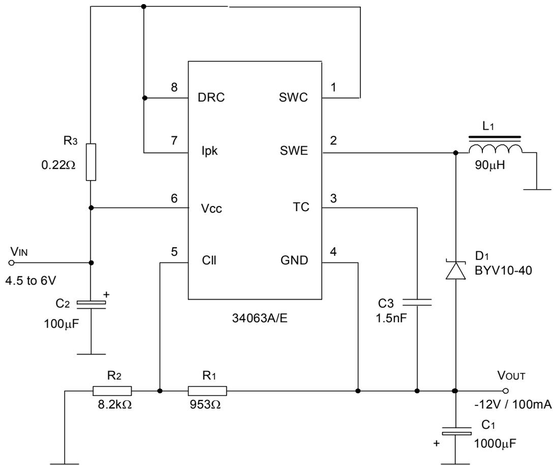
Test Condition ( $V_{OUT} = -12\text{ V}$ )
