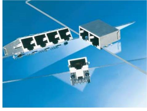
Molex introduces a new right angle modular jack with a profile of 9.53mm (.375") from the top of the PCB to the top of the jack allowing for optimal board stacking. This unique design allows the bottom of the modular jack to sit flush with the bottom of the PCB, adhering to the 2mm industry specification for creepage and clearance. The compact jack is offered in one, two and four port variations to meet many design configurations.
