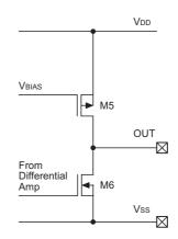
To keep power consumption to a minimum, the output short circuit current is limited to about -9mA for the source drive and 9.5mA for the sink drive. This is considered to be enough for most low power systems, however it is recommended only to used load resistors of >10k $\Omega$  for most applications. For heavy load driving applications, an external buffer stage using bipolar transistors is recommended.
