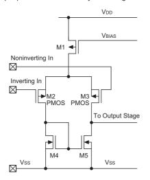
Since the input impedance of a PMOS transistor is inherently very high, they can be directly coupled to high impedance elements without loading effects. Examples could be coupling to ceramic transducers, integrating capacitors and resistor networks. It is this high input impedance characteristic that is its major advantage over its bipolar counterpart in certain application fields such as integrators where op-amp input currents can cause significant errors.
