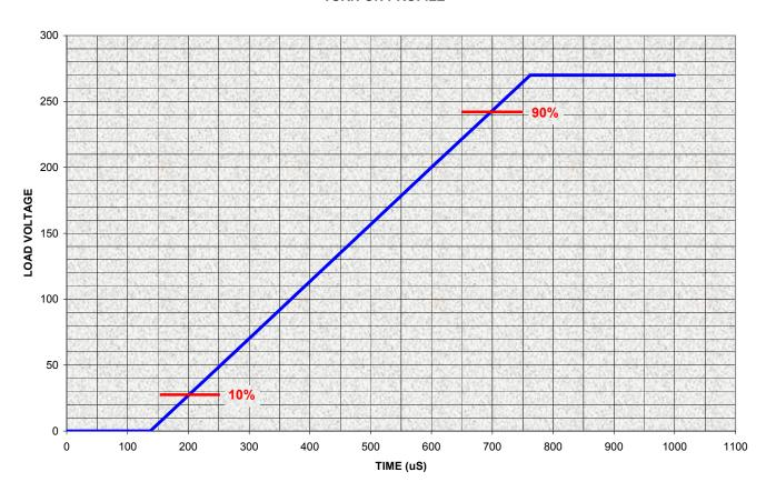
The SSPC applies Voltage to the Load at a fixed rate of approximately 43V/100uS during Turn-On independent of the Load Current. This corresponds to a Turn-On time of 500uS when measured from 10% to 90% with an applied voltage of +270VDC.
