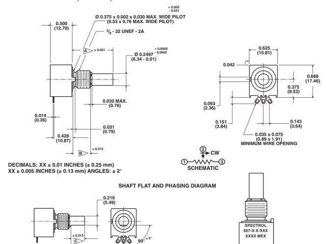
WITH SHAFT FLAT POSITIONED AS SHOWN, OUTPUT RATIO TO BE  $e/E = 0.50 \pm 0.02$
