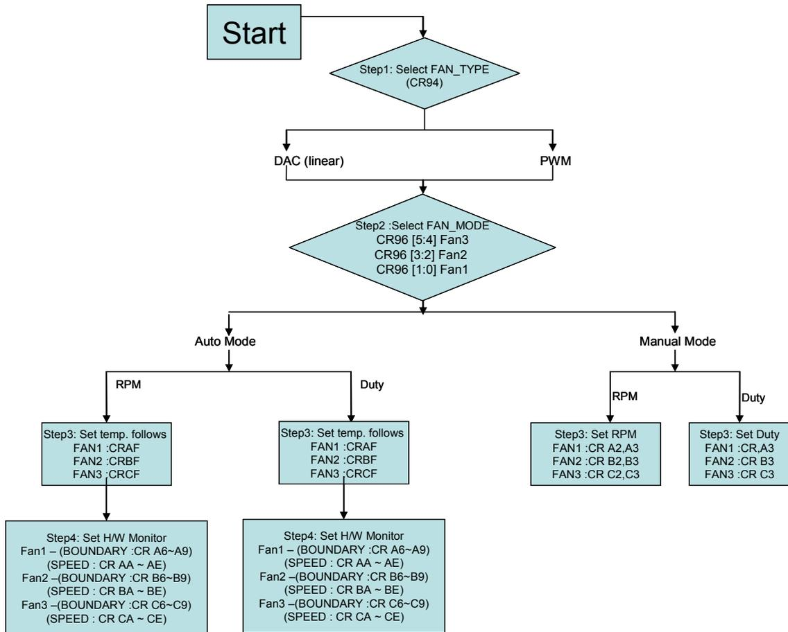
Fig 6-7 Fan type & mode selection flow
