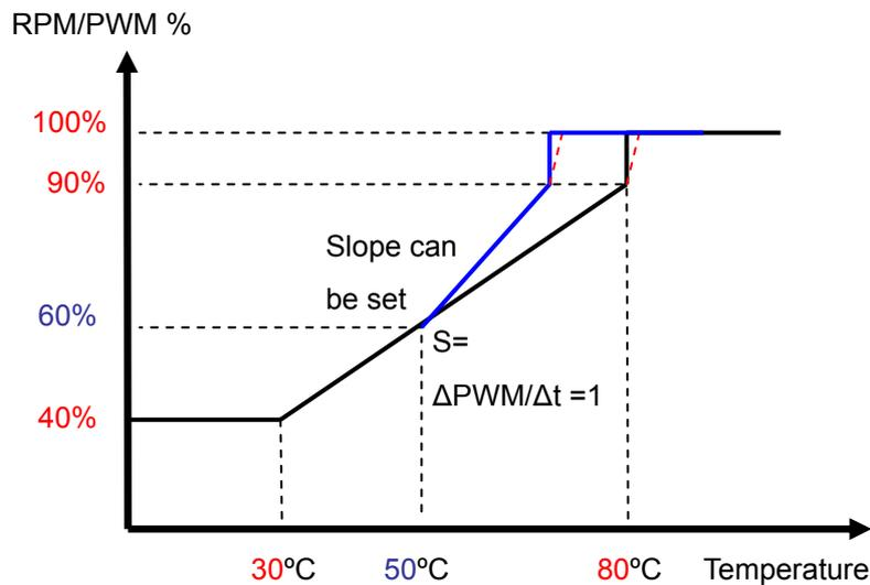
**Figure 6-13 Support 2 Linear Application with Multi-Temp. Setting**
